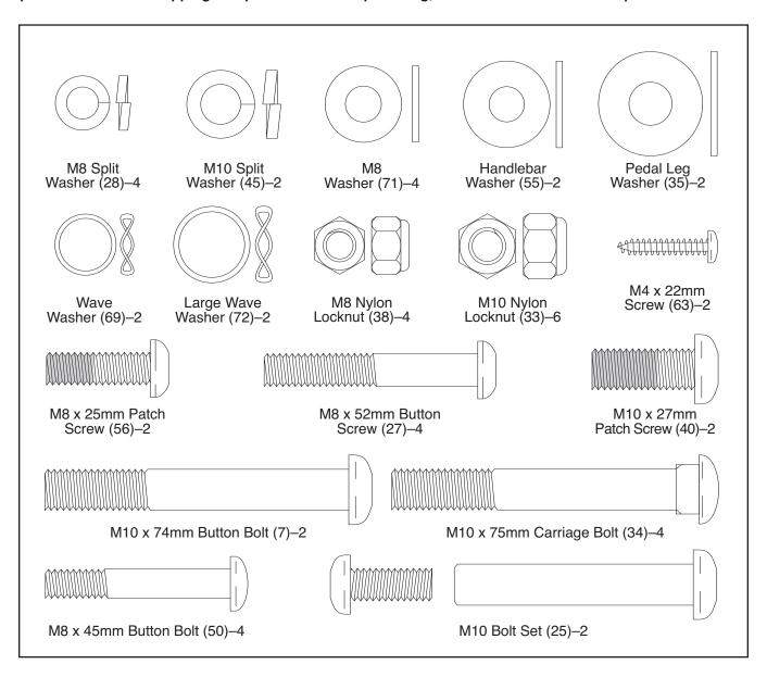
Identify the Front Stabilizer (10), which has round Endcaps (21) on its ends. While another person lifts the front of the Frame (1), attach the Front Stabilizer to the Frame with two M10 x 75mm Carriage Bolts (34) and two M10 Nylon Locknuts (33).
